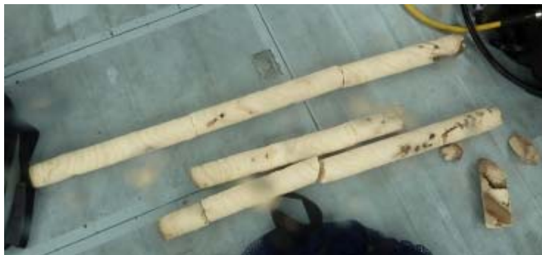
Corals grow annual density bands that can be counted like tree rings. Researchers have measured lead in coral samples shown, and traced the history of lead deposition in the Indian Ocean. Photo - Photo: Intan Nurhati
